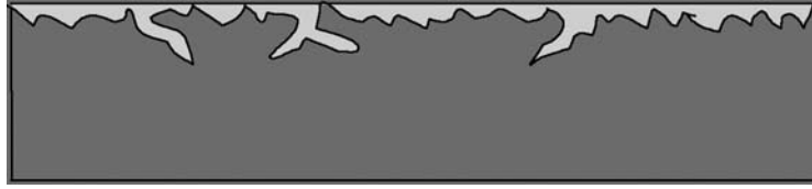
Figure 5-10. Mechanical adhesion as a result of surface roughness.
