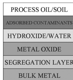
Figure 5-8. Schematic representation of a metal surface prior to surface preparation.
