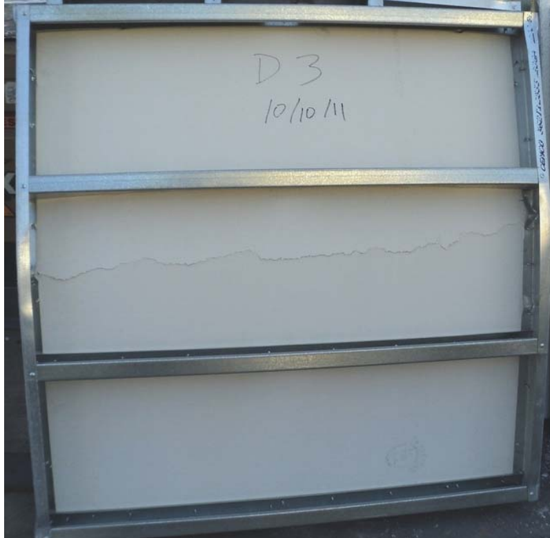
Photo 3 – Typical Failure (D3)
